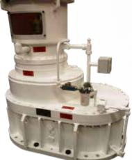
• Hofmann swing shaft assemblies can be upgraded with HofCarb pinions.
